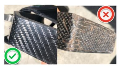
**Bucklings & Rivets**: Have not moved, not fractured / bent, different from original shape or excessively worn.
